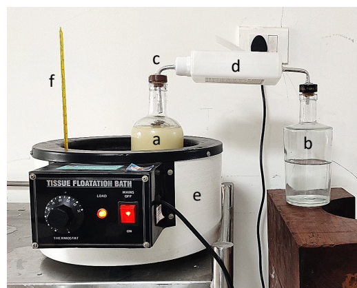
Fig. 1: Shows the cost-effective acetone reclamation setup
