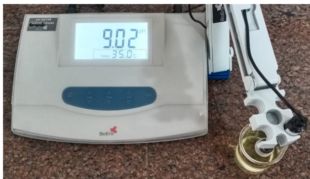
Fig. 3: Impure acetone readings in the pH meter show a pH of 9.02, which indicates a high level of impurity
